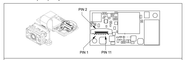
Figure 34. Decode Board (USB) Output Connector
